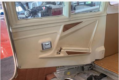
As with the Spatial Interior, fitting new foot panels with see-thru templates makes install quick and perfect. Door jamb and pilot lower panels are out of the box ready to install. Dual lock fastener assemblies are simple and work well.
