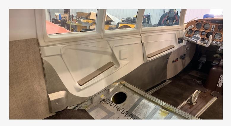
Removing the interior revealed deteriorated plastics, original fiberglass and evidence of mouse infestation. Only minor tubular rusting was a relief and plastics were repairable. Installing new closed cell foam insulation complied with a mandatory service bulletin.
