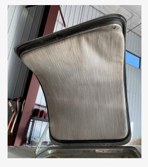
Deteriorated baggage door liner can be replaced with a new flat panel. Finishing visible metal edges creates a professional final look.
