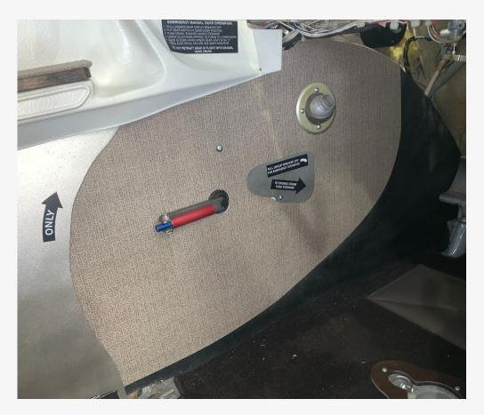
Revitalization kit includes 5 cabin and 3 baggage panels, see-through install templates, dual lock fastening assemblies and ty-raps, additional length of dual lock for shimming around wire bundles, baggage corner angle brackets, decal set, burn test documents.
