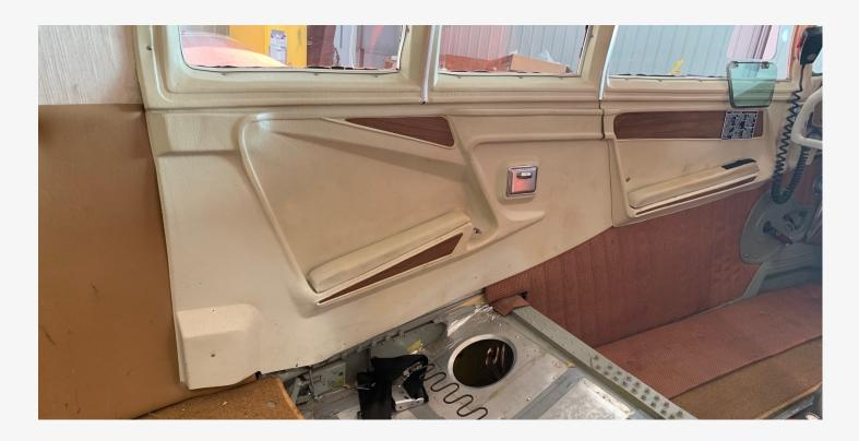
Revitalization kit includes foot, lower pilot, door jamb, spar and baggage area panels. Select fabric and colors for a fresh new look.
