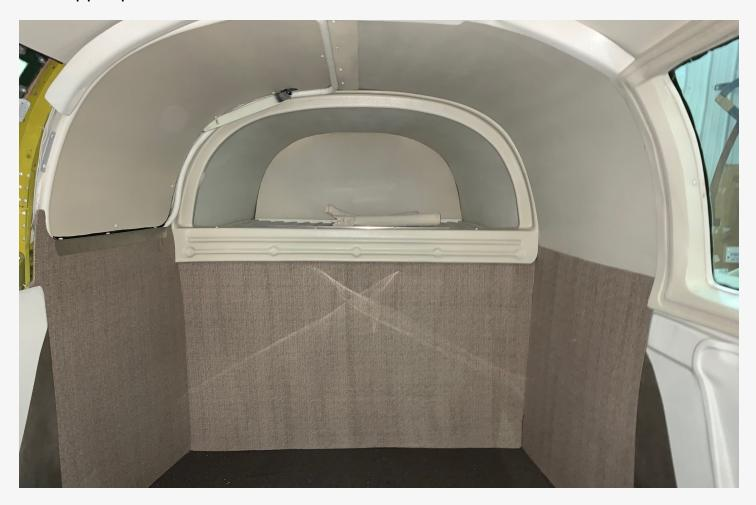
Spar panel covered with fabric and attached storage pockets is held in place with dual lock assemblies and original floor brackets.
