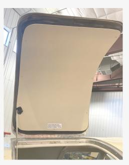
Wheel well covers can be reconditioned in place by cleaning, masking and applying finishes. Worn fuel selector fairing can be replaced with a two part assembly creating more finger room for tank selection.
