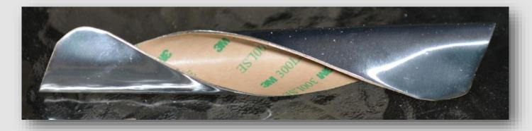
Soft aluminum .016 foil and acrylic transfer tape very effectively cover typical blemishes from pulled through screws, aging and heat damaged plastics. Cut with a scissors, this easily formed material precisely profiles to the mating surface. Turn the page for edge repair suggestions.
