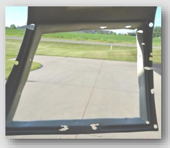
After scrub cleaning, profile every blemish with a Dremel cutting or grinding tool keeping edge openings to a minimum. Scuff underside with coarse sandpaper and clean with Plastic Prep. Apply acrylic patches to totally cover the blemish while wrapping slightly to the front side.
