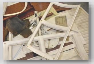
With eyeball vent headliner in place, apply plastic prep aerosol and scrub with Scotch Brite pad. Wipe with soft cloth and mask as needed. Before applying aerosol finishes, repair blemishes as described in the following pages.
