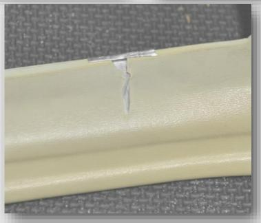
Soft aluminum acrylic tape patches form easily to cover blemishes. Wrapping around edges adds the strength to eliminate cracking again. Filled with PlasticWeld, texture and colors creates a like-new look.
